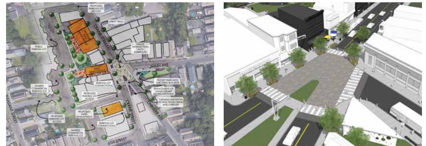
A raised intersection was proposed for the Crane-Main-Chrisler intersection in the Craig Main Complete Streets Study. While a raised intersection was the preferred solution, neighbors expressed during this project that, given the tremendous expense associated with raising the pavement, a textured solution may be more appropriate. Images Credit: Craig Main Connection Complete Streets Study
