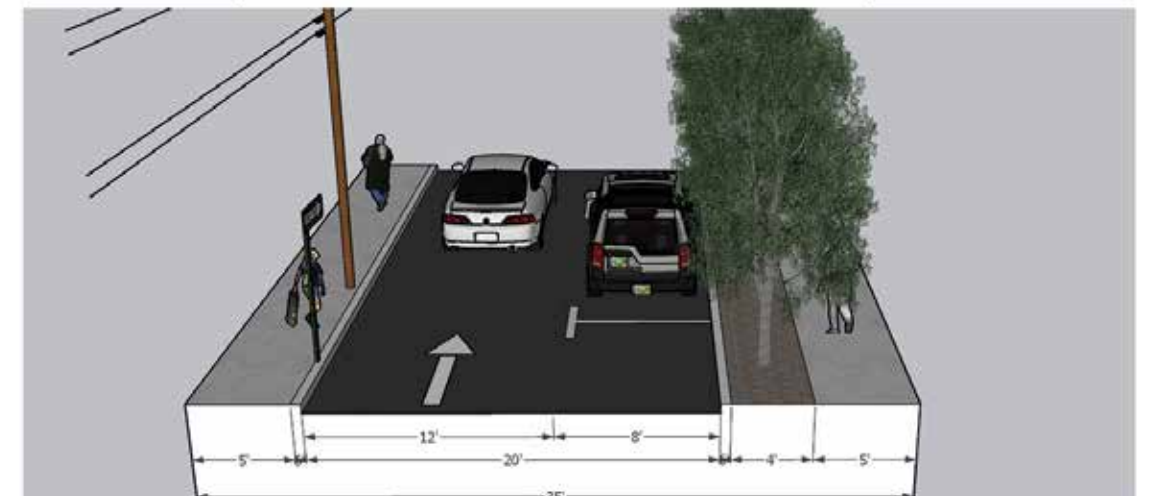
Figure 5.17: Chrisler Avenue : Main Ave to Ostrander Pl Design Concept Cross-Section All renderings, illustrations, or other mapping/imagery are design concepts and require additional engineering analysis to determine their feasibility.
