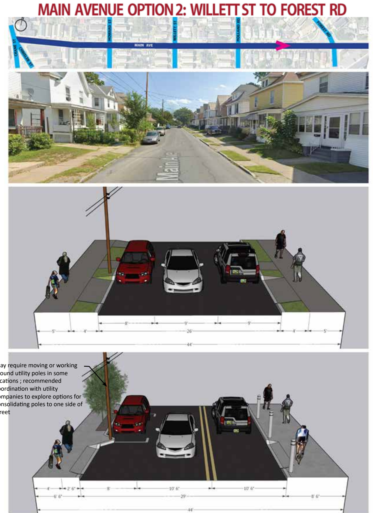
Figure 5.22: Main Avenue : Willett Street to Forest Road Design Concept 2 (Option 2) Cross-Section All renderings, illustrations, or other mapping/imagery are design concepts and require additional engineering analysis to determine their feasibility.
