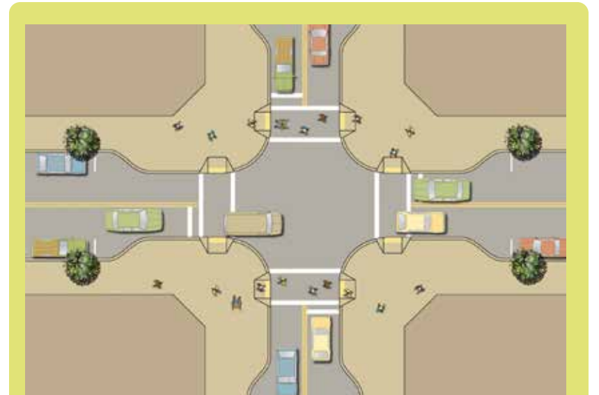
Corner Bumpouts and Cross Walks Concept Image Image Credit: Hawaii Intersections and Crossings Toolbox
