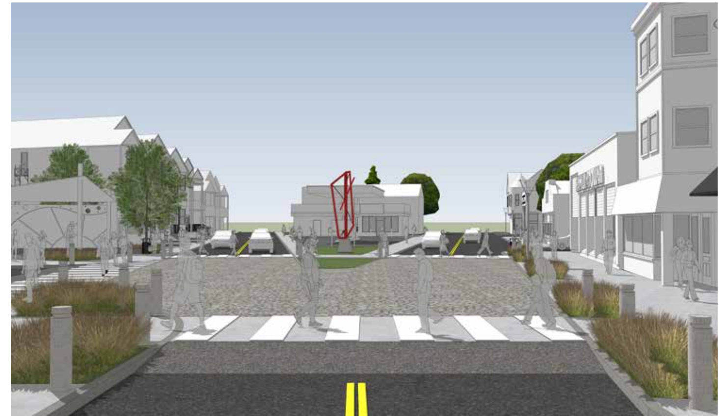
Figure 5.14: Crane Street, Main Avenue & Chrysler Avenue Intersection Concept - The Craig-Main Connection recommended eliminating parking in the intersection areas, narrowing the lanes to keep vehicles in the drive aisles, and including a raised table to encourage drivers to pass through the intersection more slowly. Image Credits: PLACE Alliance.
