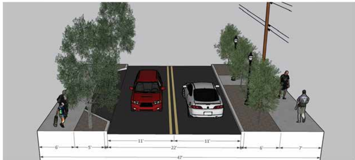
Figure 5.13: Crane Street : Main Ave to 6th Ave Design Concept Cross-Section All renderings, illustrations, or other mapping/imagery are design concepts and require additional engineering analysis to determine their feasibility.
