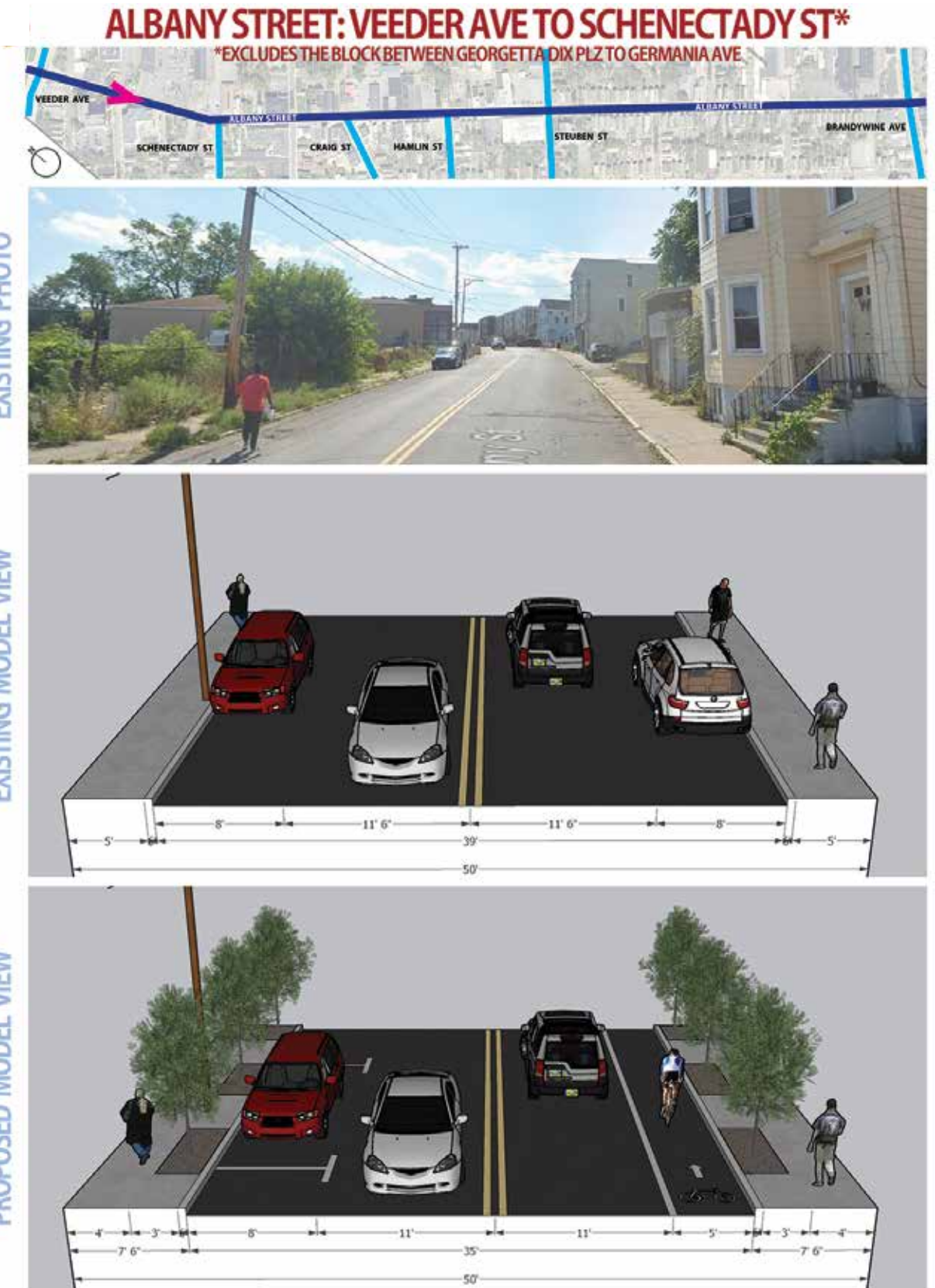
Figure 5.3: Albany Street : Veeder Ave to Schenectady St Design Concept Cross-Section All renderings, illustrations, or other mapping/imagery are design concepts and require additional engineering analysis to determine their feasibility.
