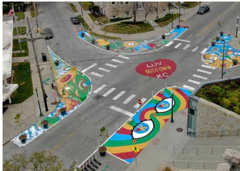
Painted Bumpouts with Seasonal Elements Concept Image Image Credit: Bloomberg Philanthropies Asphalt Art Initiative
