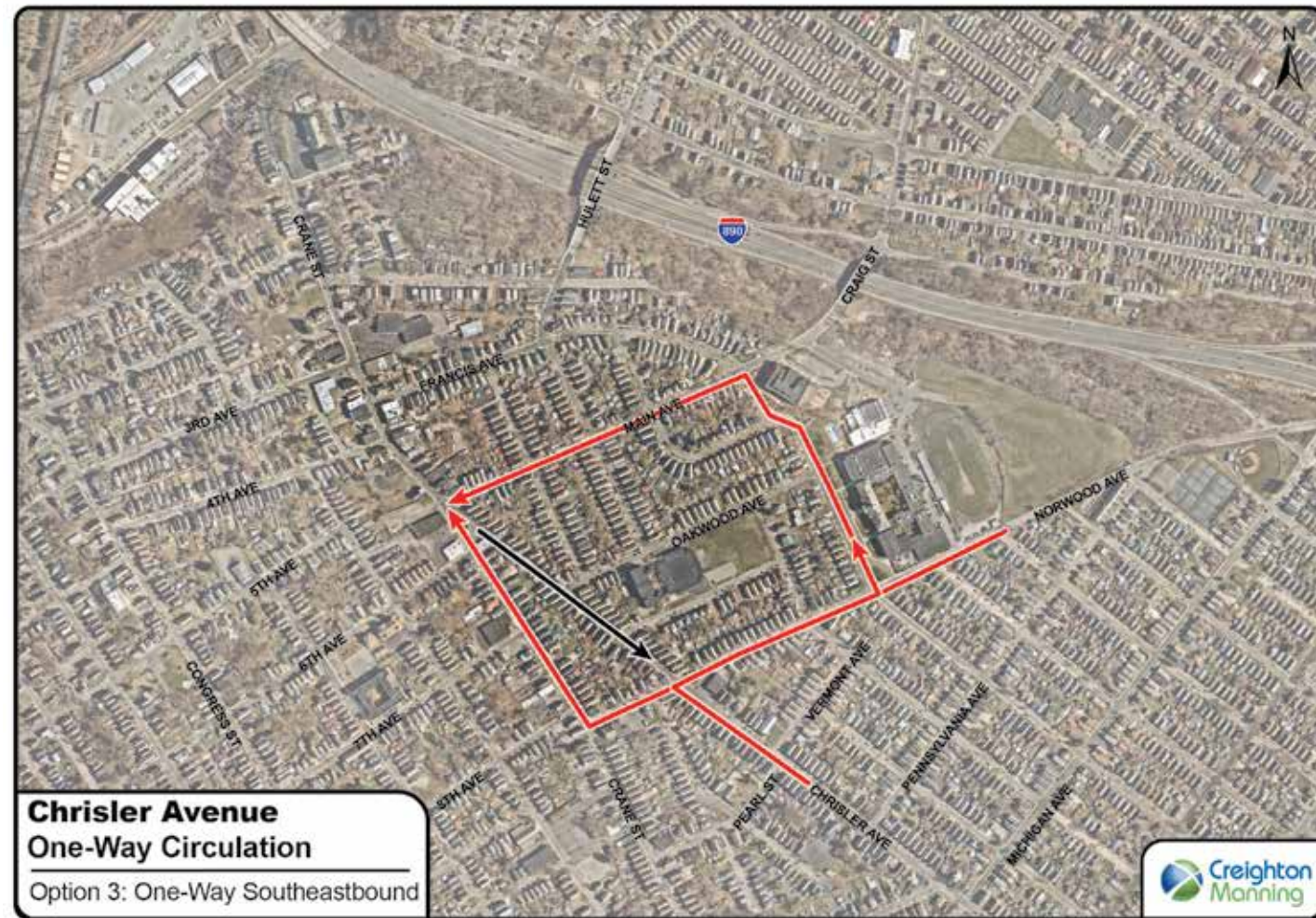
Figure 5.18: Chrisler Avenue : Main Ave to Ostrander Pl Concept Diagram Showing One-Way Circulation Southeastbound All renderings, illustrations, or other mapping/imagery are design concepts and require additional engineering analysis to determine their feasibility.
